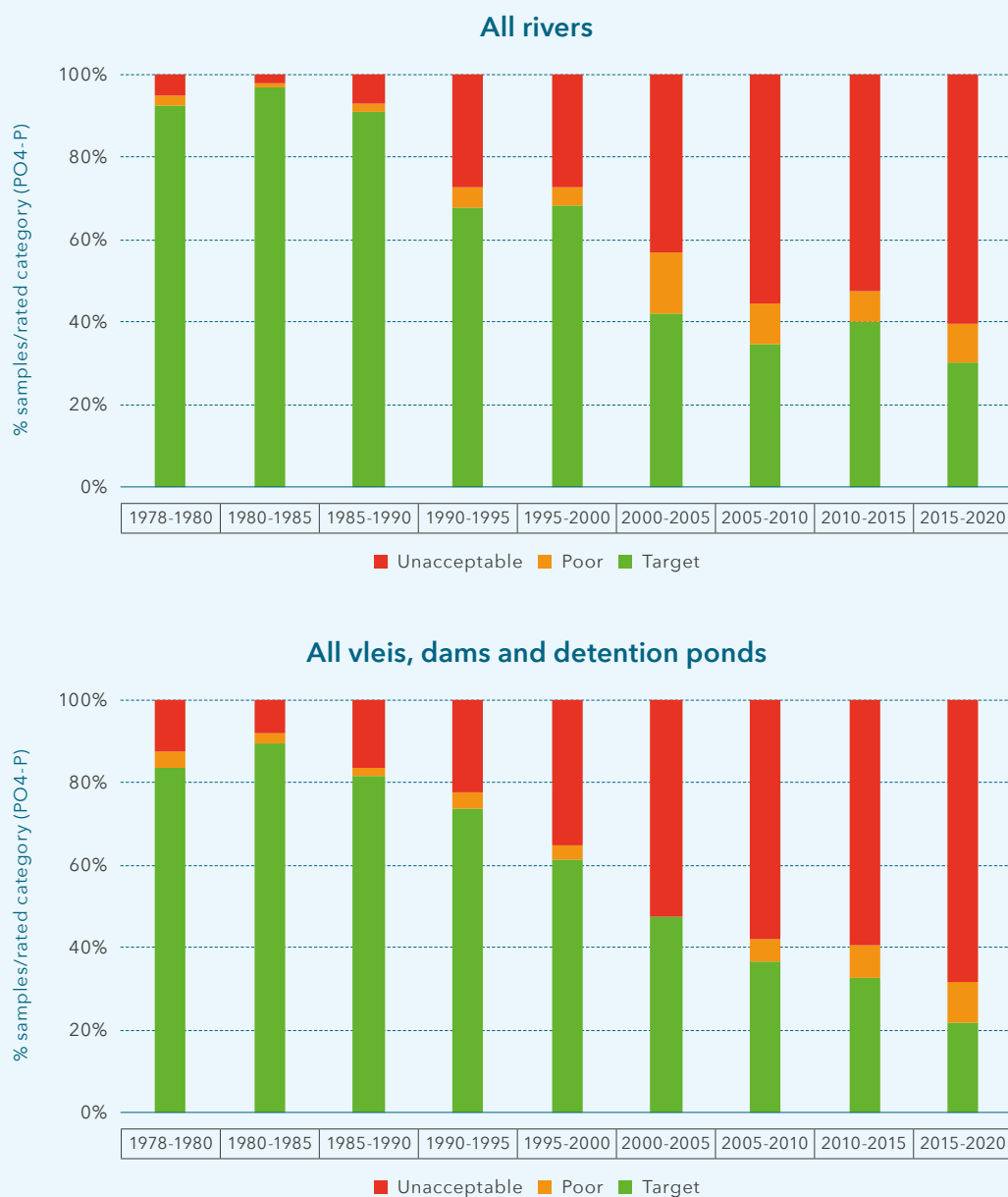
FIGURE 7: LONG-TERM TREND IN PHOSPHORUS ENRICHMENT AT RIVERS AND VLEIS/DAMS, 1978-2020
